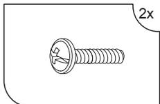
2x<br>Винт M4x16 мм          |
